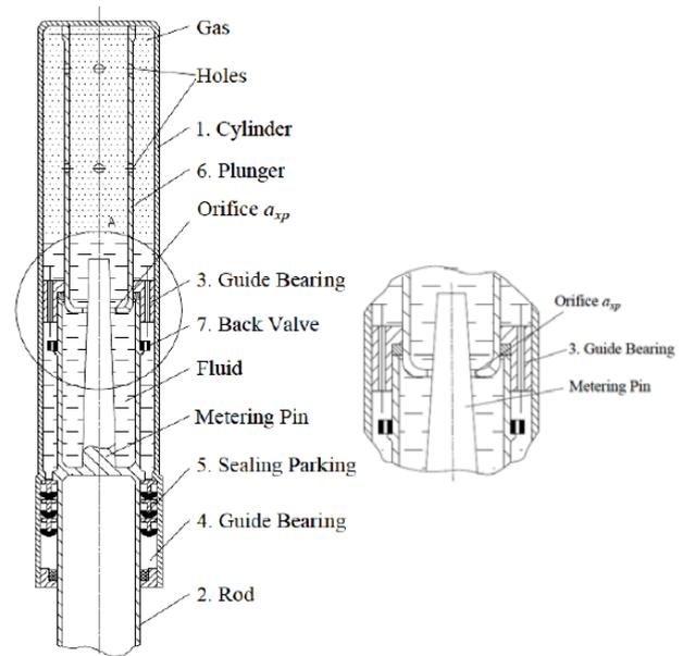
Figure 1. Schematic diagrams of passive shock absorber with metering pin
