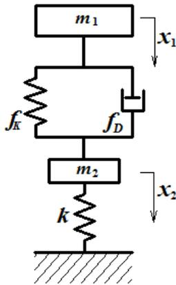
Figure 3. Model of an aircraft landing gear
