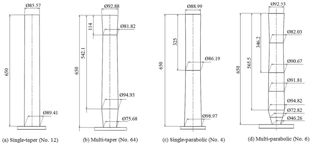
Figure 13. Metering pin diagrams of optimal solutions examples
