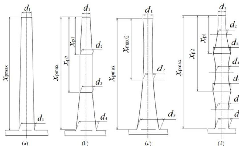
Figure 2. Schematic diagrams of the metering pin constructions
